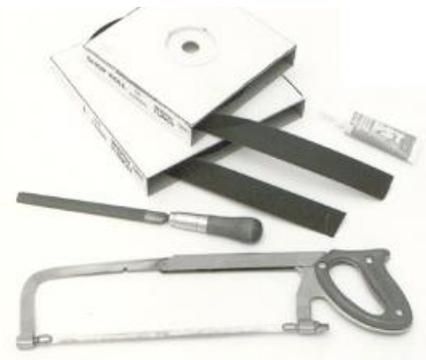
**Figure 5: Accessories for Pipe/Tube Preparation**
