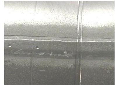
**Figure 17: Seam Misalignment**
