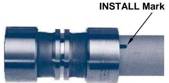
**Figure 35: Pre-Installation Process**
