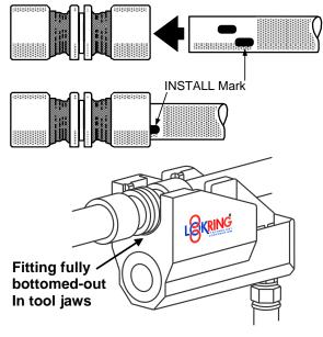
**STEP 5:** Carry out visual checks below to verify successful installation.
