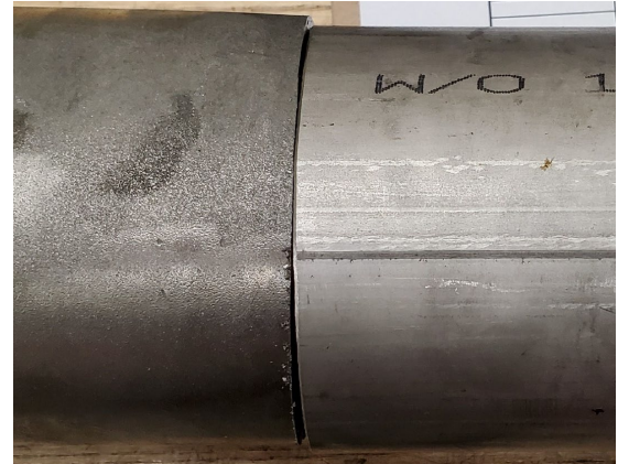
Figure 18b: Surface imperfections from sandblasting pipe OD surface (on left). Pipe on right is as supplied pipe OD surface.
